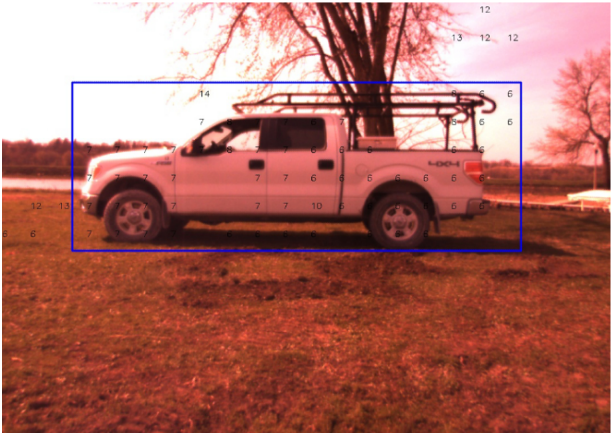
Figure 4.2 The Result After The Blood Fill Algorithm When One Foreign Object (vehicle) Is in Front of The Camera
